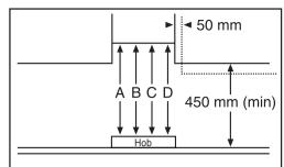
A: Built-in Electric Hob: 650mm minimum clearance
